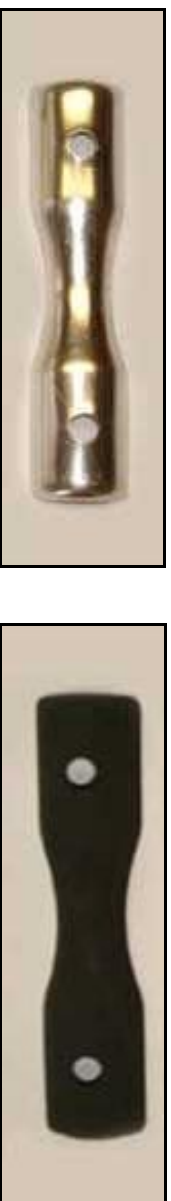
Figure 51 : Shiny metal surface left and blackened metal surface right
