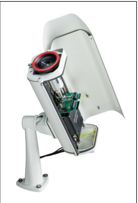
Figure 20: Outdoor protective housing for Xi camera
