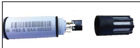
Figure 28 Filter Cap Removal
