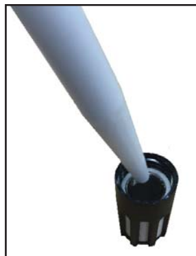
Figure 29 Filter Element Cleaning
