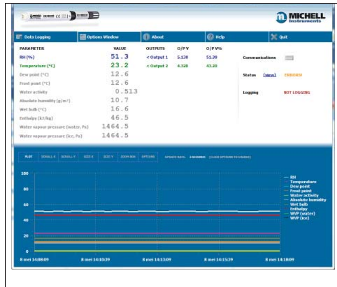
Figure 20 Probe readings prior to adjustment
