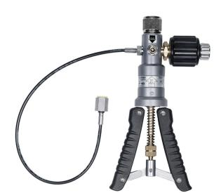
The PGS40 is a 3 in 1 calibration hand pump for vacuum, low and medium pressure replacing 3 conventional hand pumps. It is capable to quickly generate from -960 mbar to 40 bar with minimum effort. The ergonomically de-signed moulded handles provide perfect grip and comfort even when generating high pressure. The PGS40 hand pump can be supplied as pump only or as part of a pressure test kit with a large selection of BSP, NPT and Metric adapter and all in house hard transit case.
