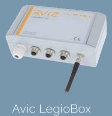
The LegioBox BasicGate is Avic's all-round IoT device for stand-alone operation in industrial environments. It can be powered either from universal AC mains or 24 VDC, supported by an internal back-up battery. The LegioBox BasicGate can either connect to a local area network (Ethernet), or through cellular networks using its 2G/3G or LTE modem. The LegioBox BasiGate supports a multitude of industry-standard process interfaces, as well as data communication ports.
