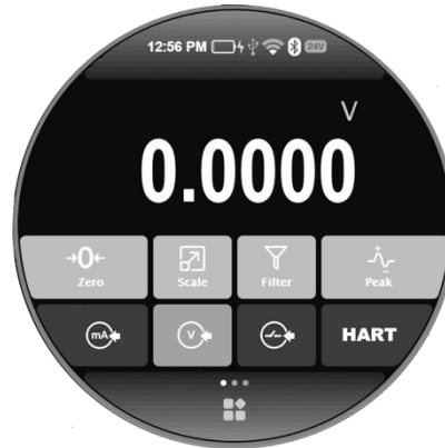
Figure 6 Electrical signal measurement function
