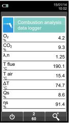
**Automatically saves** the second sample when the set time is over and so on until the last sample.
