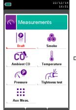
ACQUIRE THE FOLLOWING MEASUREMENTS BEFORE PROCEEDING WITH THE COMBUSTION ANALYSIS (see section 12.0):
