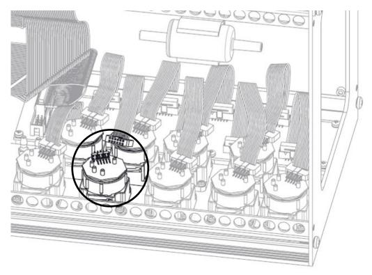
6 After rotating the sensor, pull it upward; here is an example of the sensor compartment with a sensor removed.
