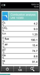
Automatically saves the second sample when the set time is over.
