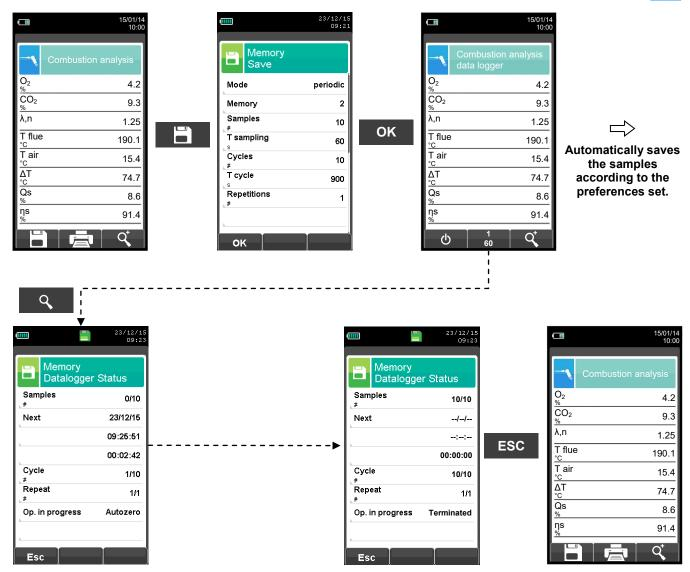
NOTE: Once the emissions analysis is completed (an audible signal will be emitted), the average of the samples acquired will be displayed on the instrument.
