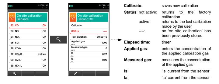
4. In the following is described in detail a recalibration example for CO sensor.
