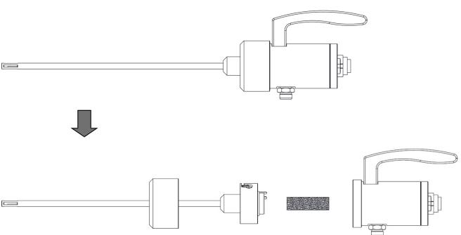
• To reassemble the probe logically reverse this procedure.
