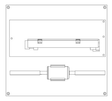
An infrared bench for the detection of gases based on (NDIR) infrared spectroscopy can be installed on **CHEMIST 900**. By this system it is possible to simultaneously detect CO, CO2 and CxHy.
