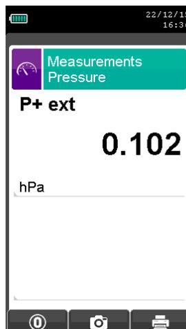
Measurement of the pressure by means of an external micromanometer.
