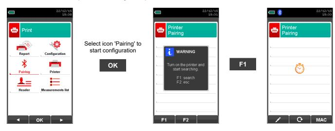
2. Select the line corresponding to the desired Bluetooth printer, then proceed as follows:
