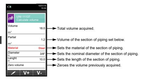
Adds up the volume of the section of piping entered.
