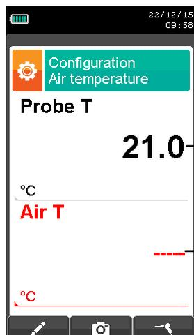
21.0 → Combustion air temperature detected by the Tc-K probe connected to the T1 connector. If the probe is not connected, a sensor error is displayed.
