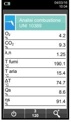
Automatically saves the third sample when the set time is over.
