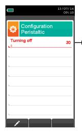
➤ Power-off time configurable in the range 30 .. 3600 seconds.
