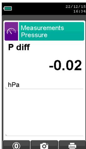
Measurement of the differential pressure by means of the internal pressure sensor (piezoresistive, temperature compensated).
