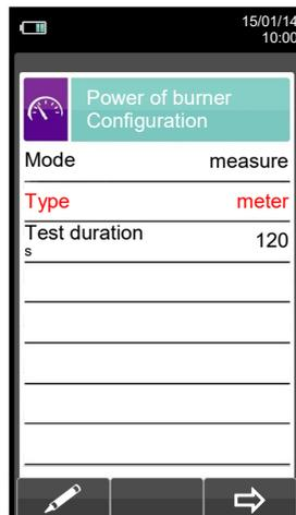
Test mode: you can choose to calculate the thermal power by entering a flow value, or by reading the volumetric counter (gaseous fuels only).
