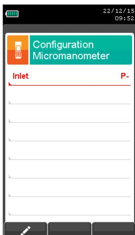
→ Sets the input used for the test: P+ or P-
