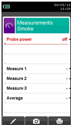
→ When manual pump kit is used set to ' off ' the probe power supply.
