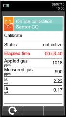
Zeroes the timer helps to keep under control the time elapsing during the stabilization phase.
