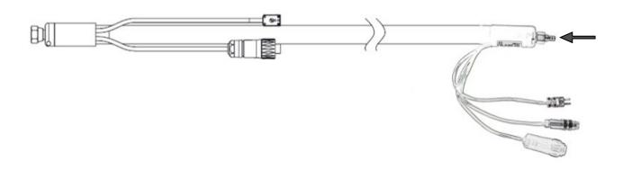
• Clean the filter in an ultrasonic bath or by using solvents and steel wire brushes.
