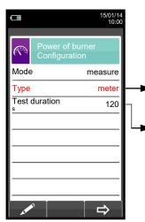
Test mode: you can choose to calculate the thermal power by entering a flow value, or by reading the volumetric counter (gaseous fuels only).
