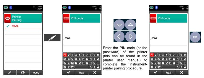
3. The instrument-printer pairing is completed. Press key ' [ESC] ' to return to the previous screen.
