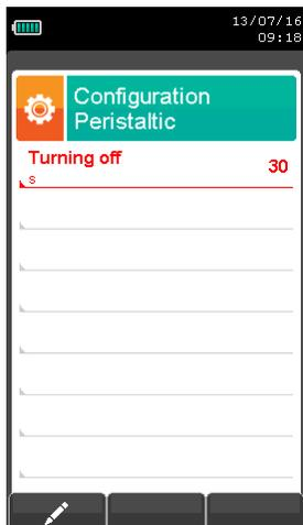
→ Power-off time configurable in the range 30 .. 3600 seconds.
