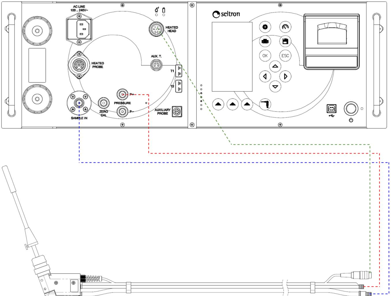
Heated head probe for smoke measurement: (AASX04 / AASX05).
