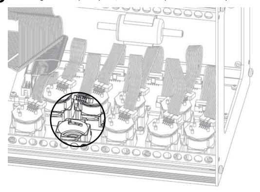
6 Fit the new sensor again taking care the electric connection is turned to the outside the instrument, not the inside (See point 4).
