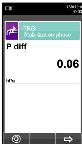
12.10.3 Performing a tightness test for a gas line with volume greater 200 liter.
