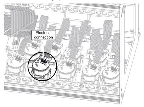
3 Disconnect the sensor to be replaced; here is an example of a disconnected sensor to be replaced (the electrical connector has been disconnected).
