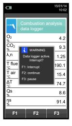
**Automatically saves** the first sample when the set time is over.
