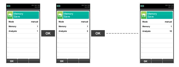
Example 2: Saving the combustion analysis in automatic mode (example UNI 10389)
