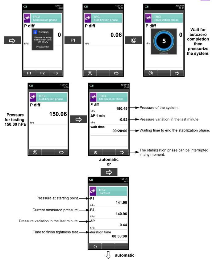
NOTE: If, while configuring the tightness test the automatic printing mode has been selected, the tightness test is printed automatically.
