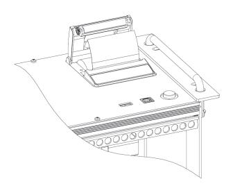
Close the whole block of the lid of the printer, pressing it lightly so as to hook it on to the device.
