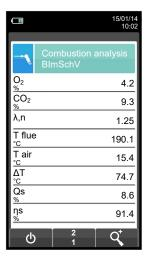
Automatically saves the second sample when the preset time interval has elapsed and so on until the last sample.
