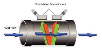
Transducers ultrasonic signal path Transit-time flow measurement technique
