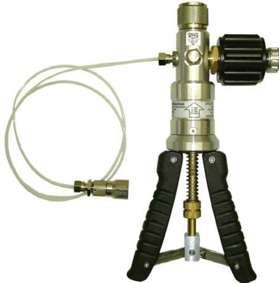
PGS-40, max. pressure 40 bar vacuum -0.95 bar
