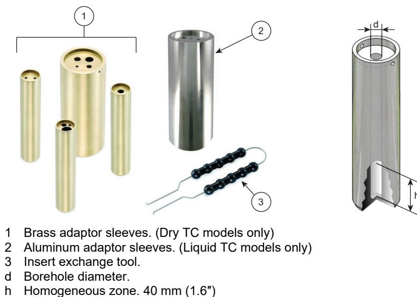
Figure 3: Adaptor Sleeve Inserts
