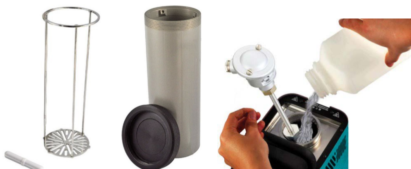
Figure 13: Filling with Calibration Liquid
