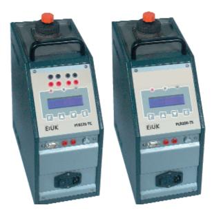
The PLB series are portable liquid baths (Portable Temperature Calibrators) designed and manufactured by Eurotron, a market leader in temperature calibration. Stirred liquid baths are suitable for calibrating temperature sensors of all size and diameters an shape without the need of specifically drilled block. They also provide much smaller calibration uncertainty than Dry Blocks.
