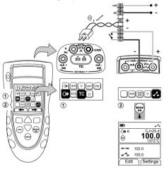
Figure 12: Example configuration - Switch test
