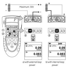
Figure 3: Example configuration - To measure mA (Dual Function, area <sup>(2)</sup>)
