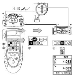
Figure 2: Example configuration - To supply mA with internal loop power (Area <sup>①</sup>)
