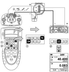
Figure 11: Example configuration - Transmitter calibration with internal loop power
