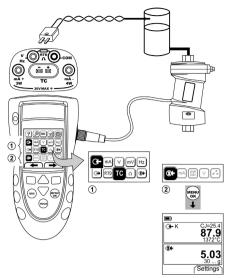
Figure 14: Example configuration - To measure pressure and temperature
