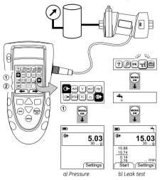
Figure 13: Example configuration - Pressure measurement with a UPM
