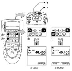
Figure 6: Example configuration - To measure/supply Hz or Pulses
